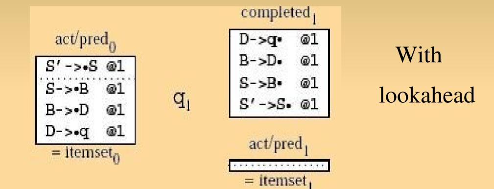
Earley Parser shows a very successful combination of strong sides of top-down and bottom-up methods, handles well left recursion and  $\varepsilon$ -rules, and, being armoured by lookahead, takes the optimal possible amount of memory.
