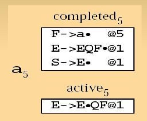
S --> E● @1 is in the set completed and the last input symbol has been read.
